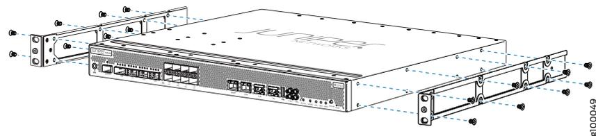
4. Install the two front ETSI brackets on the front-mounting brackets on each side of the chassis (see [Figure 27 on page 68](#)).
